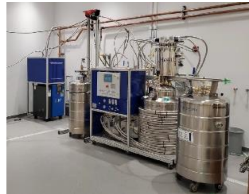
Liquefier & cryostat in LH 2 configuration
