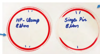
Figure 8. Red fuji film showing load on DIN 32676 gasket caused by single-, and double-pin clamp.
