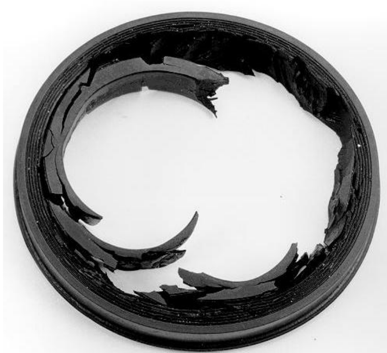
Figure 9 Complete disintegration caused by RGD
