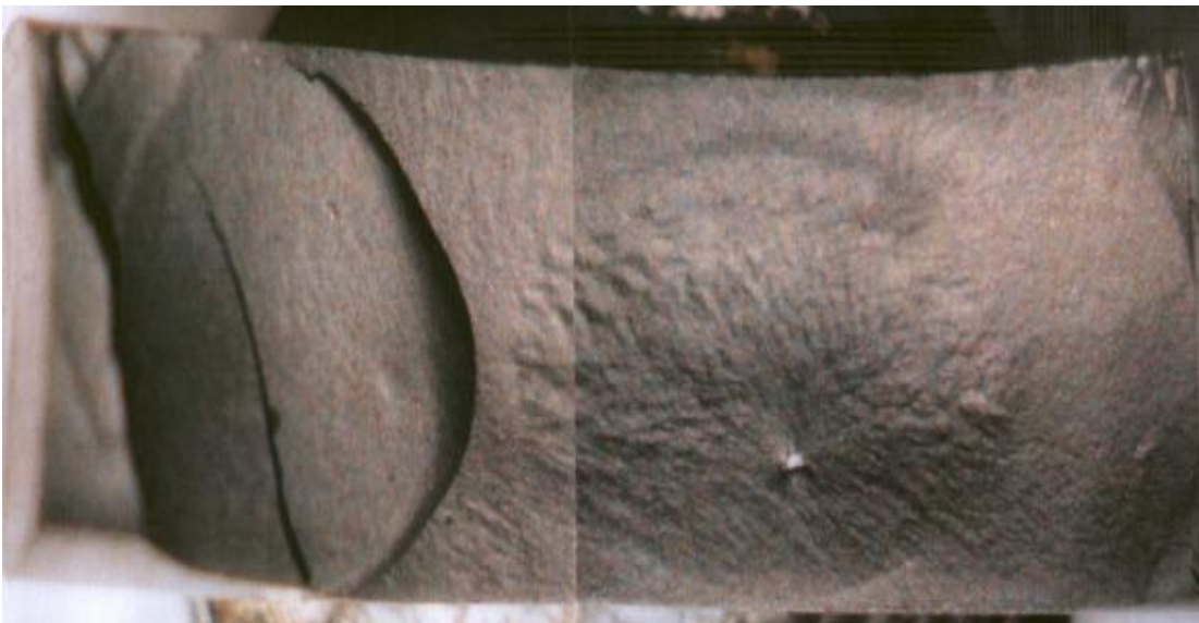
Figure 11 RGD fracture initiated by inclusion (external contaminants or undispersed compounding ingredients)
