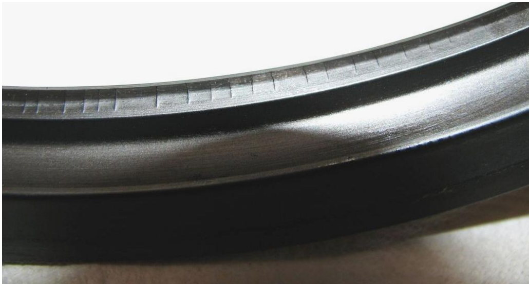
Figure 19: Cracking on lip seal
