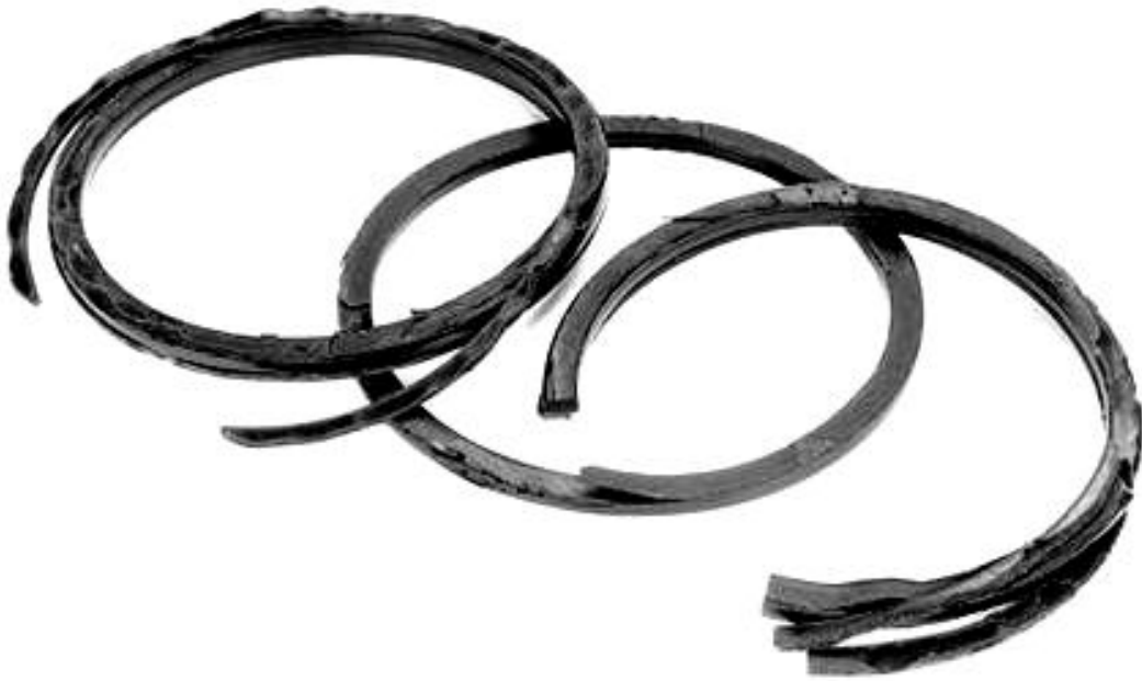
Figure 36 Air entrainment causing fabric delamination on a piston seal
