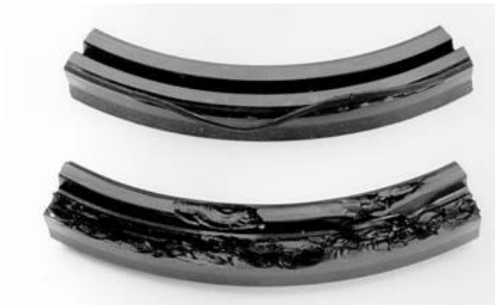
Figure 40 Seal damage caused by inter-seal build up
