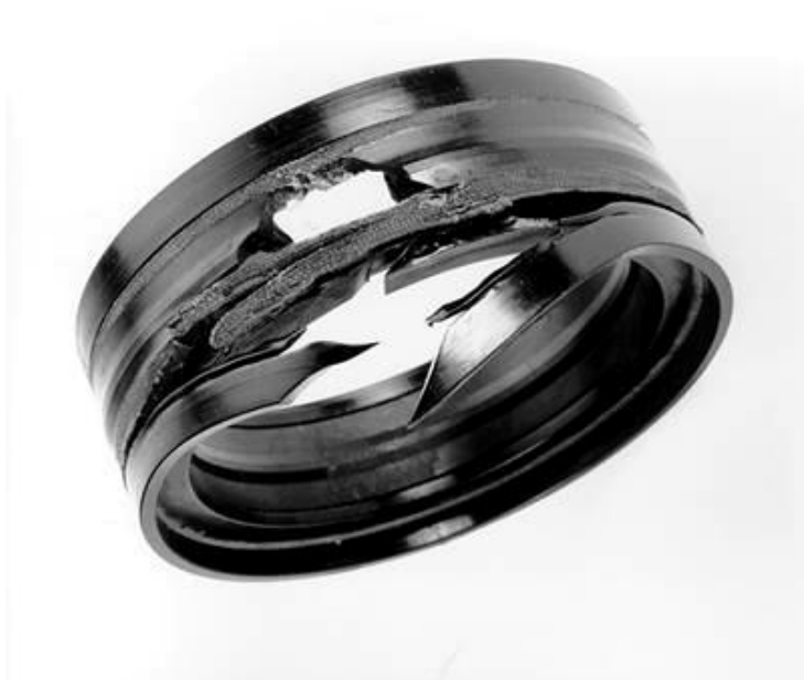
Figure 35 Catastrophic seal failure caused by dieseling
