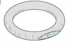
Figure 28 Skive damage due to traversing port
