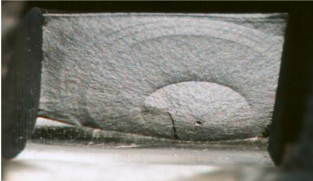
Figure 10 RGD fracture initiated at void
