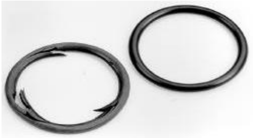
Figure 8 Splitting caused by RGD
