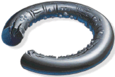
Figure 5 Rapid Gas Decompression
