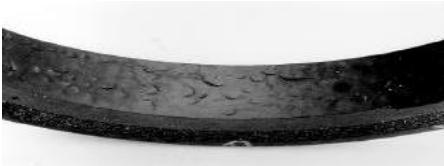
Figure 6 Blistering caused by RGD
