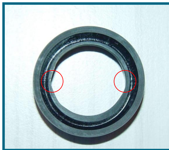
Figure 44 Uneven wear of a lip seal
