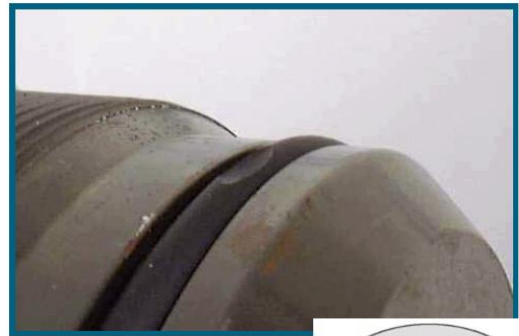
Figure 28 Skive damage due to traversing port
