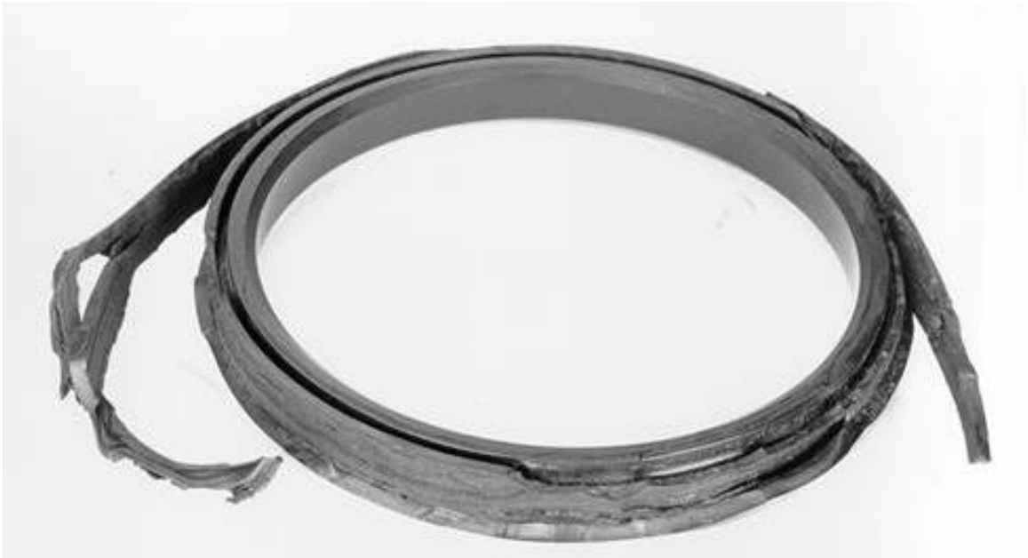
Figure 41 Seal damage caused by inter-seal build up
