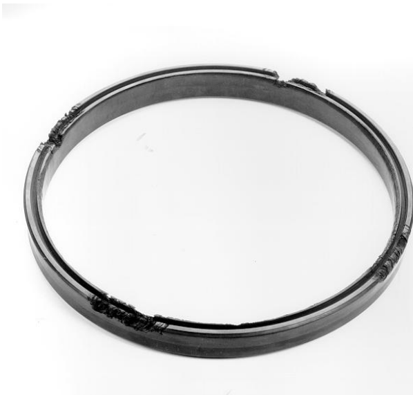
Figure 29 Seal damaged by connection holes
