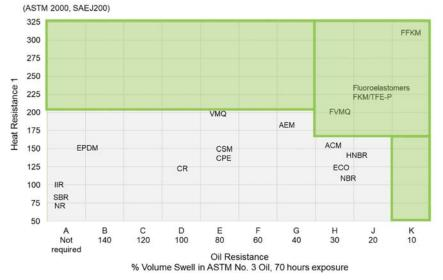
$^1$  Maximum temps at which vulcanizates can be aged for 70 hours with changes in tensile strength  $\leq \pm 30\%$ , elongation  $\leq -50\%$  and hardness  $\leq \pm 15$  points  $\approx \pm 15$  points  $\approx \pm 10^{-1}$  points
