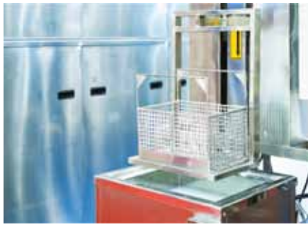
Ultrasonic cleaning of seals.
