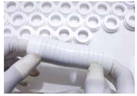
Visual inspection of seals.
