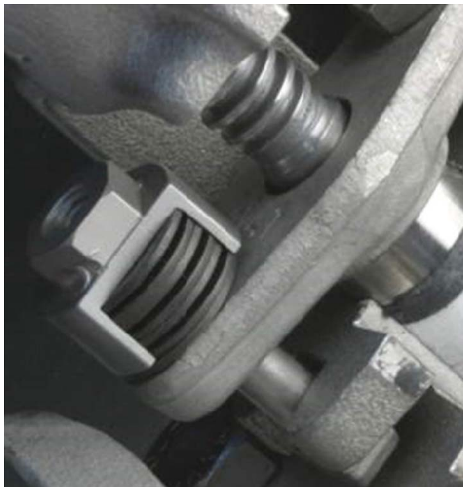
Fig. 2: Disc Spring loaded bolt with housing (Source: Co. EagleBurgmann)
