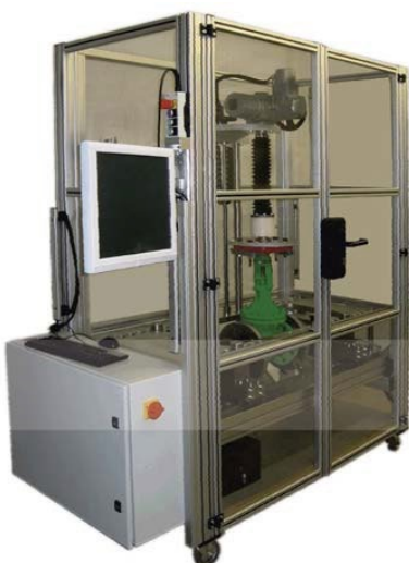
Testing equipment TEMESvalve.teq for ISO 15848-1 tests.
