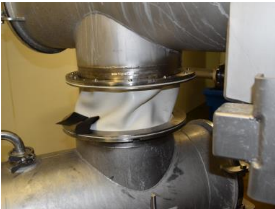
Figure 2: Prototype of new quick lock system in application
