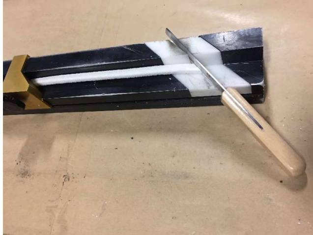
Figure 37 Measuring and Cutting Tool for Compression Packing
