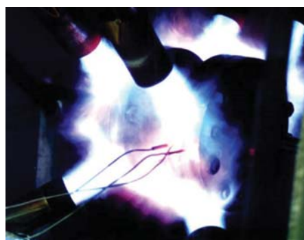
Fig 2: Exxon-modified API 607 gasket fire test.
