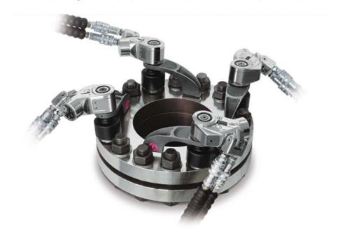
cally actuated tools are used. The use of such instruments increases the tightening speed and for this reason, they are preferred in industrial applications, due to time-saving. Hydraulic wrenches are also favored in those heavy-duty applications where extreme torques are required.
