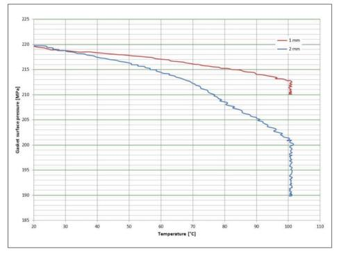
Chart 2: Changing of gasket surface pressure after loading of gasket.
