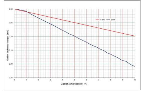
Chart 1: Gasket thickness change versus gasket compressibility.
