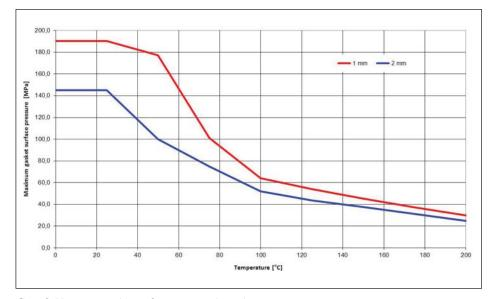
Chart 3: Maximum gasket surface pressure depending on temperature.
