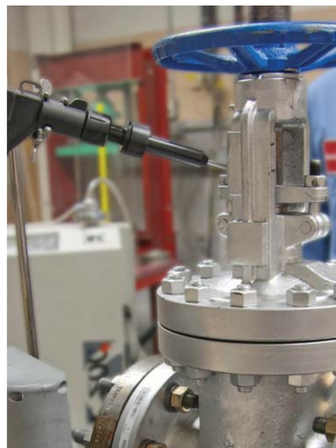
Both standards specify 'sniffing' to monitor leakage when testing with methane
