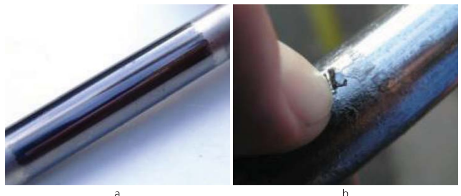
Figure 2: Graphite adhesion on the surface of the stem a) thin graphite film, b) thick graphite layer.
