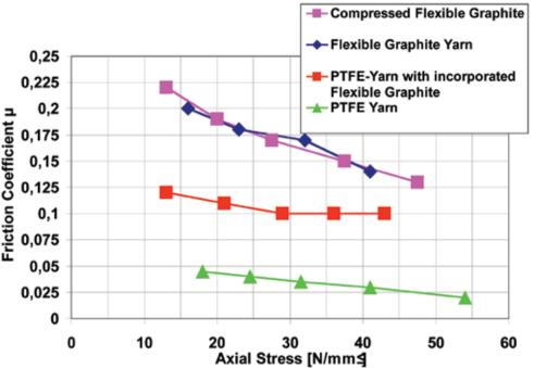
Typical friction coefficients of different packing materials at room temperature
