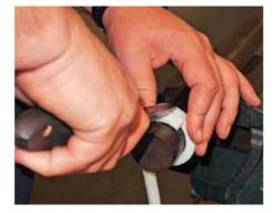
Cutting on a mandrel using "skive cut" 45° angle.
