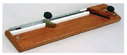
Cutting tool (ruler on top and a bench for knife on right).
