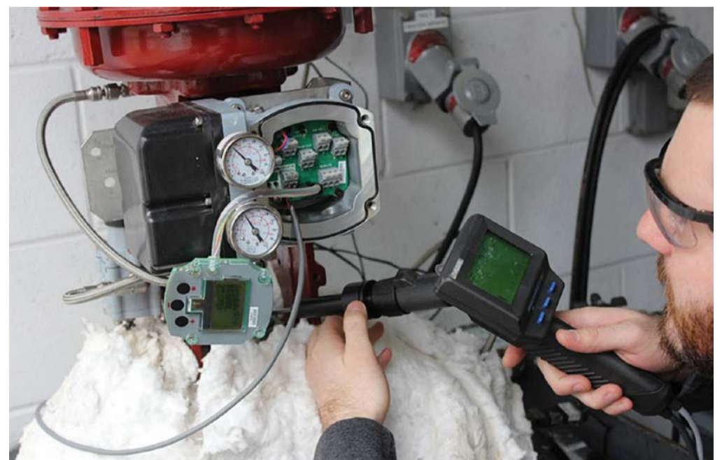
Valve testing to ISO 15848. Image courtesy of the Fluid Sealing Association
